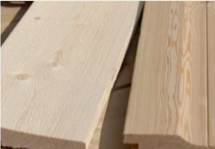
Coatings perform better on a sawn finish (left) rather than a smooth planed surface (right).
